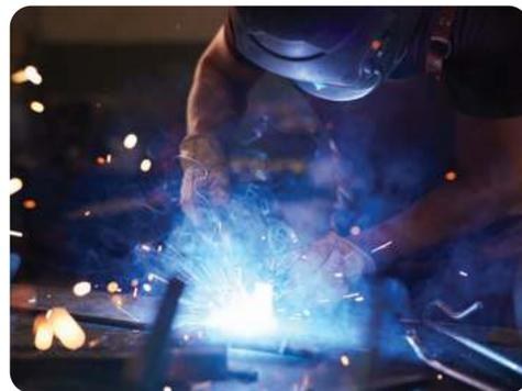
**FCAW (Flux Core Arc Welding)**
