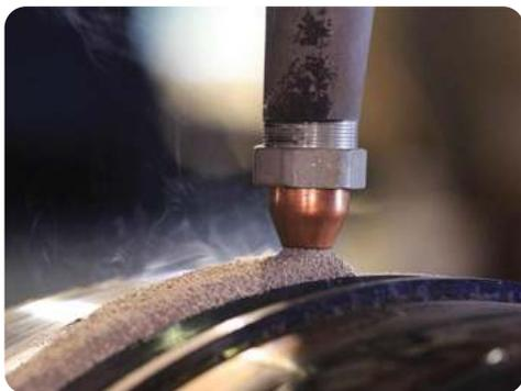
**SAW (Submerged Arc Welding)**
