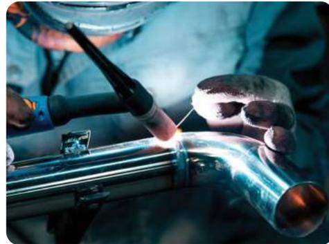
**GTAW (Gas Tungsten Arc Welding)**
