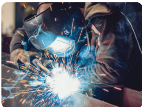
GMAW (Gas Metal Arc Welding)
